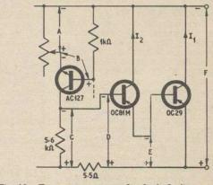
Fig. 10. Test measurements for fault-finding
