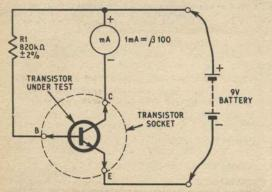
Transistor test-rig. Note: reverse battery Fig. 3.10. connections and milliammeter for pnp
