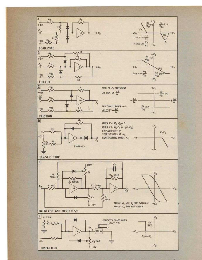
Fig. 10.2. Special circuits for simulating mechanical phenomena
