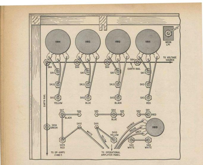
Fig. 2.4. Right-hand portion of front panel viewed from rear, showing components and wiring. Operational Amplifiers 2 and 3 are wired exactly as "Operational Amplifier 1" shown here
