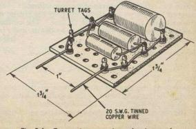
Fig. 5.4. Computing capacitor plug-in panel
