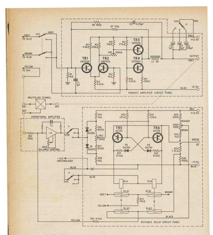
Fig. 9.2. Multiplier circuit, comprising product amplifier panel and bistable relay panel
