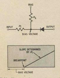
Fig. 1.4a (left). Illustrating how a mathematical function can be constructed from a series of straight line tangents Fig. 1.4b (above). A single diode network and its output characteristic
