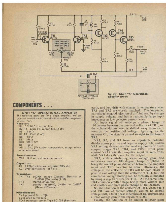
Finally, the addition of an emitter follower stage provides the low input impedance required for driving a variety of useful loads, without unwanted circuit complications. TR5 causes negligible further voltage shifting, adds no change of phase, and with a voltage gain very close to unity, will simply reduce the output impedance of the operational amplifier without modifying its other characteristics.
