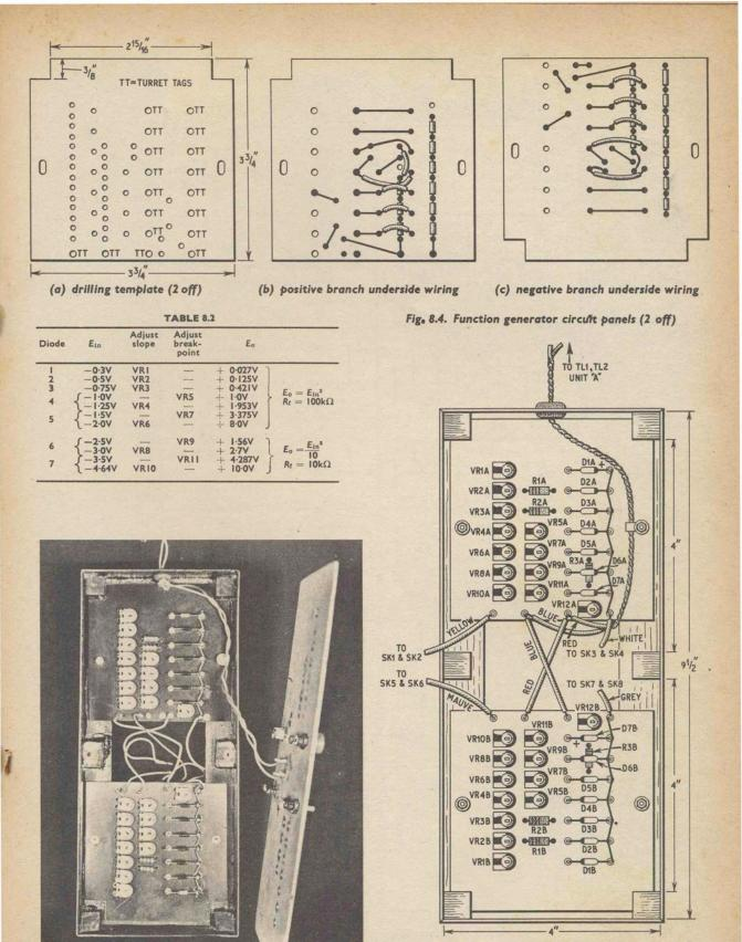
Fig. 8.5. Topside and interconnecting wiring of function generator panels. The circuit boards are shown in position inside the UNIT "C" case
