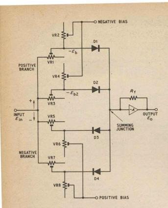
Fig. 7.8a. Circuit of a simple function generator
