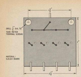
Fig. 6.8. Meter resistor panel, underside view
