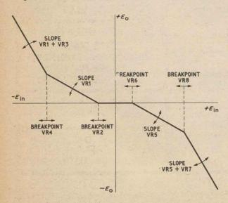
Fig. 7.8b. Adjustable characteristic of simple function generator
