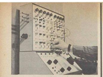
This photograph shows PEAC being used to solve simultaneous equations
