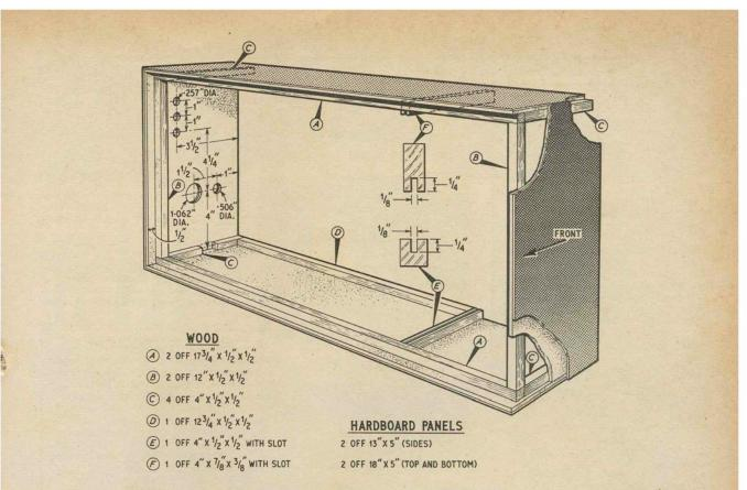
Fig. 2.12. Constructional details of UNIT "A" Box
