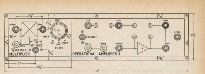
Fig. 9.3. Dimensions and engraving details for UNIT "D" front panel
