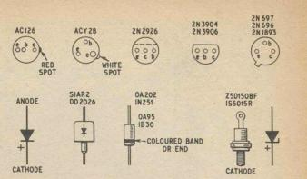
Fig. 3.3. Transistor and diode key
