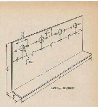
Fig. 6.6. Mounting bracket for pre-set potentiometers
