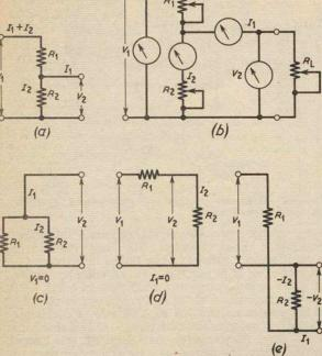
Fig. 4.4. (a) voltage divider circuit; (b) direct simulation of (a); (c), (d) and (e), three variations on (a)
