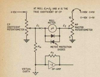
Fig. 6.4. Master potentiometer circuit for measuring coefficients
