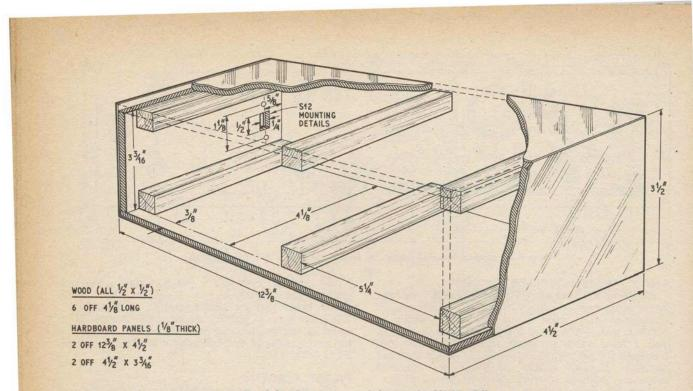
Fig. 9.4. Construction of the box for UNIT "D"
