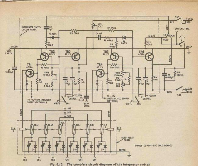
rig. o.iv. The complete circuit diagram of the integrator swit
