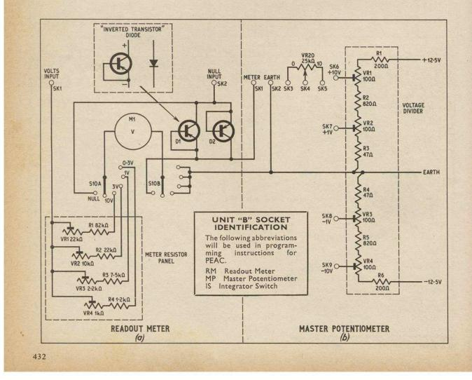
reverse characteristic. The arrangement eliminates the need for a meter series resistor while still giving adequate protection.
