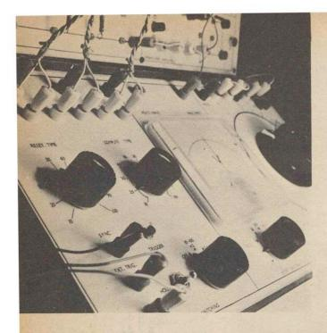
on its blocks, and, following Fig. 6.10 and Fig. 7.3, wire all controls and sockets to the turret tags on the two sub-assembly panels, again with p.v.c. covered flexible wire, long enough to allow the switching circuit panel to be turned over for underside inspection. Run red and blue wires from S9, and a green wire from IS/SK12, to the power pack output solder tags, and fit knobs to S9, VR18, and VR19.
