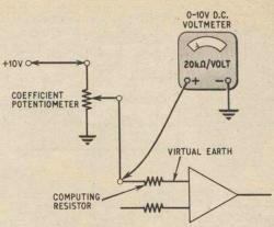
Fig. 4.3. Voltmeter method of determining coefficient potentiometer settings
