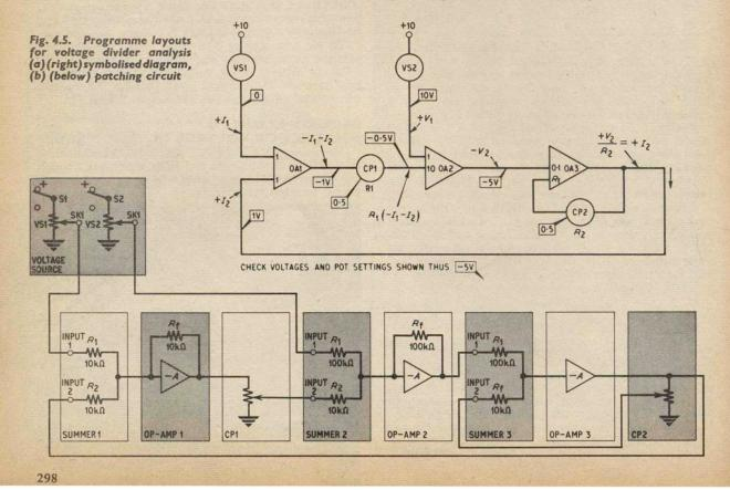
terms of Eq. 4.5  $(I_2)$ . To see how the problem is set-up on the computer, refer to Fig. 4.5, and note the changes of sign involved.
