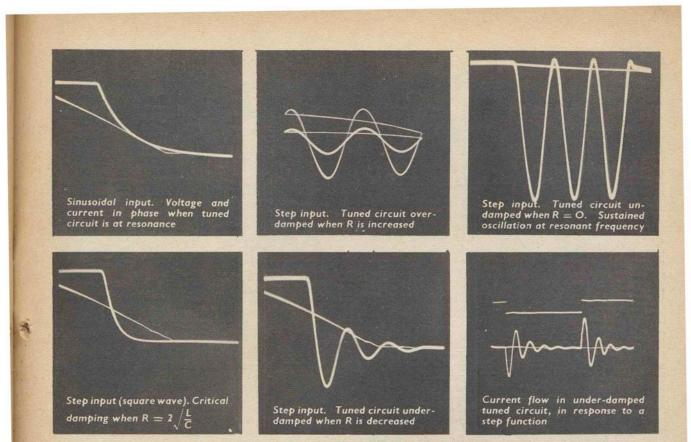
Fig. 5.7. Response of a simulated tuned circuit
